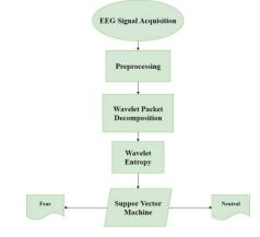
Figure 3. Flowchart of the signal processing methodology.
