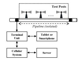
Figure 1. The LWSN-based Monitoring System [15].
