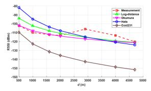
Figure 6. Comparison of the measured and simulated data (rural).
