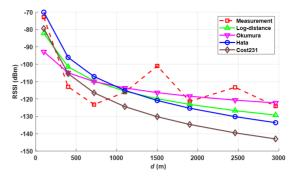
Figure 7. Comparison of the measured and simulated data (suburban).
