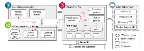
Figure 8. A possible hardware deployment for E-HoA architecture
