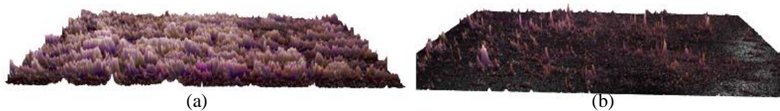
Figure 9. Digital Image of (a) Unpolished and (b) Polished Surface of 10 mm Cube Specimen
