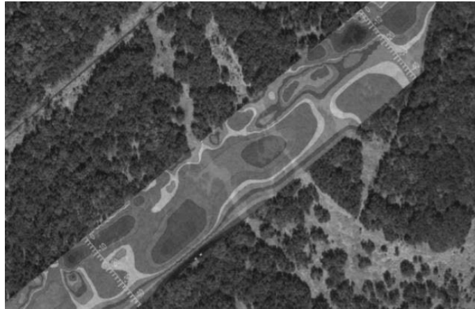
Figure 3. Aerial photo of Bracken Bat Cave Preserve with an overlay of the previously performed resistivity study. Photo taken from Green (2008).
