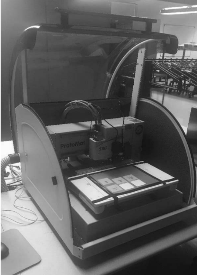
Fig.1. LPKF ProtoMat S103: photograph of device used to fabricate macro- and microscale test sections
