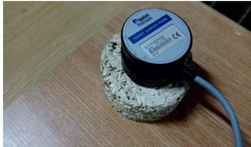
Figure 7 – Measuring the heat transfer coefficient
