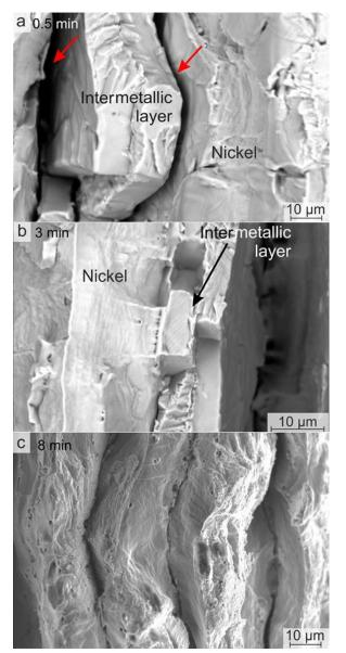
**Figure 8** Fracture surface the Ni-Al MIL composites sintered by SPS for 0.5 (a), 3 (b), and 8 (c) min.
