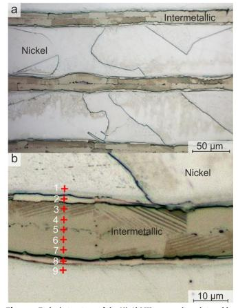
**Figure 4** Etched structure of the Ni-Al MIL composites sintered by SPS for 3 min: overall cross-section view (a); structure of the intermetallic layer in the cross-section (b). The point numbers correspond to the numbers of the EDX spectra (Table 2).
