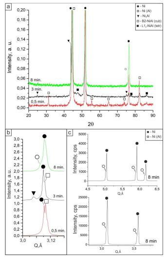
**Figure 1** X-ray diffraction patterns of the Ni-Al MIL composites obtained by SPS for 0.5, 3, and 8 min: X-ray diffraction patterns recorded using diffractometer (a); X-ray diffraction patterns in Q of the peak corresponding to  $2\theta$  range  $\sim$ 38–47 degrees from the patterns in Figure 1a (b); X-ray diffraction patterns recorded using synchrotron facility (c).
