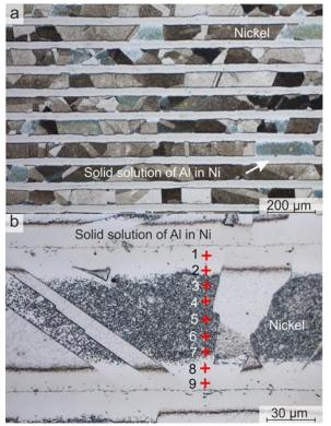
**Figure 5** Structure of the Ni-Al MIL composites sintered by SPS for 8 min: (a) overall cross-section view; (b) structure of the intermetallic layer in the cross-section. The point numbers correspond to the numbers of the EDX spectra (Table 3).
