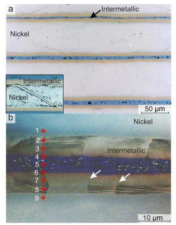
**Figure 2** Structure of the Ni-Al MIL composites sintered by SPS for 0.5 min: overall cross-section view (BF mode) (a); the etched structure (inset); structure of the intermetallic layer in the cross-section (DIC mode) (b). The point numbers correspond to the numbers of the EDX spectra (Table 1).
