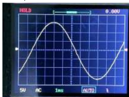
Figure 3: Output Waveform of Pure Sine Wave Inverter
