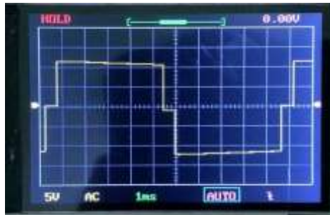
Figure 4. Modified Sine Wave Inverter Output Waveforms
