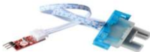
Figure 4. Turbidity Module Sensor
