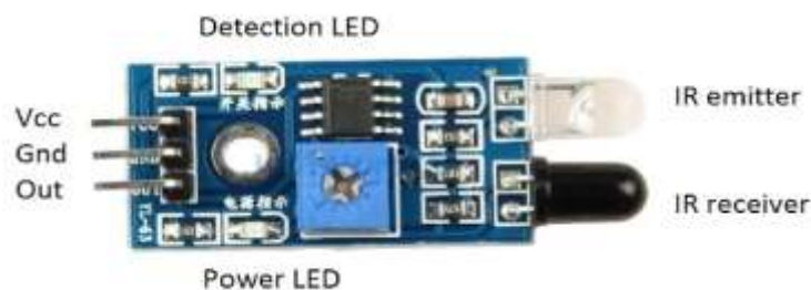
Figure 3. Sensor Proximity fc-51
