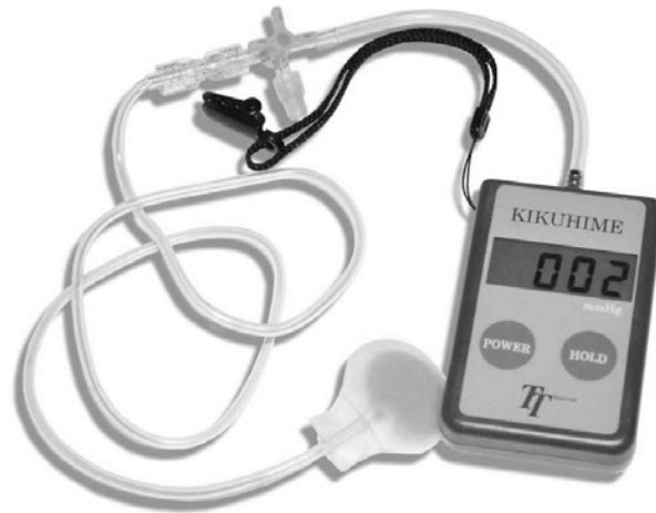
3 4 5 6 7 8 9 10 11 Figure 3.3 Kikuhime pressure sensor, adapted from Varodem (2018).
