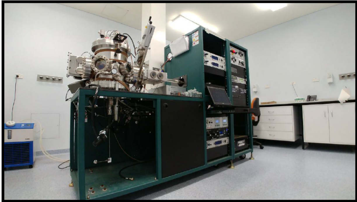
Figure 7-1. AJA Orion 5 Magnetron Sputterer used in this project. Located at Western Sydney University, Hawkesbury Campus.
