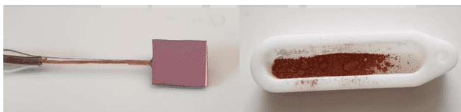
Figure 5-6. Ta_3N_5 thin film mounted as an electrode (left) and red Ta_3N_5 powder (right), reacted from Ta_2O_5 powders via thermal annealing in NH_3 .
