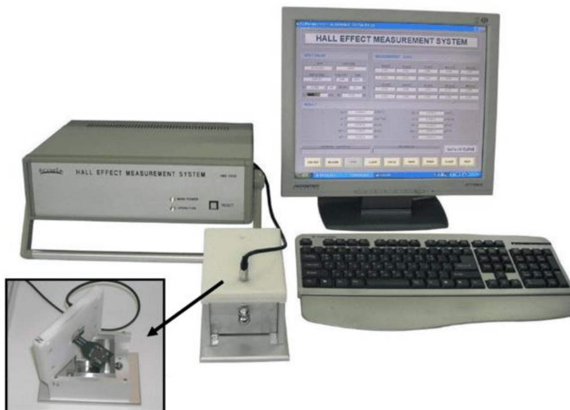
Figure 7-7. Ecopia HMS-3000 Hall Measurement System used in this project with accompanying PC and software shown. The sample mount, with mounted sample and magnet, can be seen in the bottom left.
