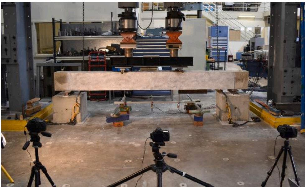
Fig. 6. DSLR cameras setup for DIC analysis.
