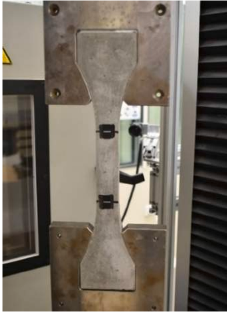
Fig. 21. Uniaxial tensile test of SPH-ECC dog-bone specimen.
