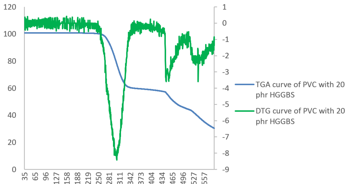
Figure 5-22 TGA and DTG curves of PVC stabilised with 20 phr HGGBS
