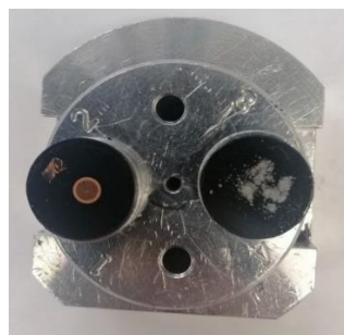
Figure 3-7 Sample preparation for SEM-EDS analysis (left: copper standard, right: ash related to one of the samples)
