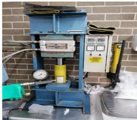
Figure 3-14 Plastic heat press machine of APN compounding
