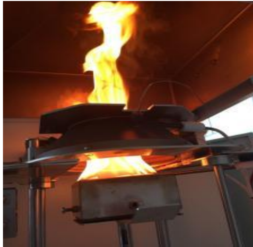
Figure 2-8 A photo of a cone calorimeter (source: Suzhou Yangyi Vouch Testing Technology Co., Ltd)
