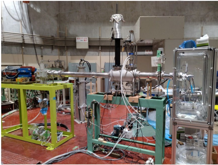
Beam course for RI production
