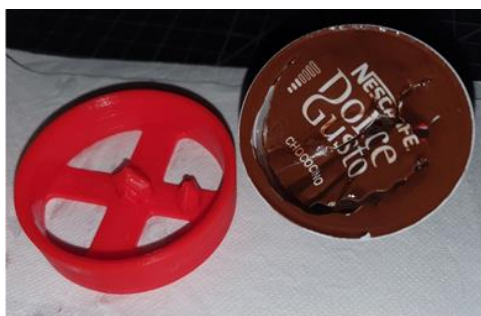
Dolce Gusto pod drainer (separates coffee grounds from container, for environmentally friendly waste processing)
