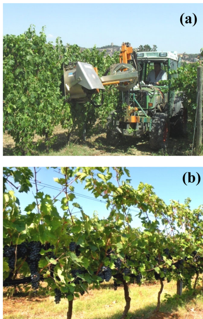
Figure 1. (a) Mechanical leaf remover operating in the Sangiovese vineyard and (b) the window opened in the canopy above the bunch zone.
