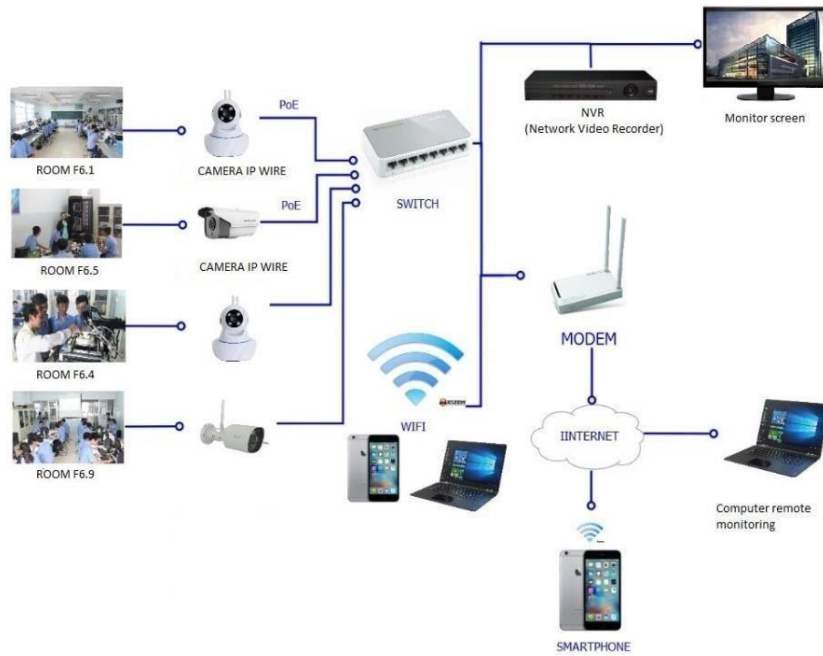
Figure 1.1: Smart monitoring system [1]
