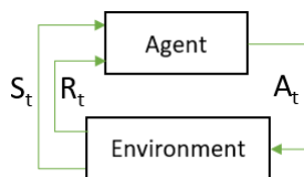
Figure 1: MDP: A learning system called an Agent inside an MDP environment, at time t observes a state s_t , selects an action a_t and receives from the environment a reward r_t then moves into the next state s_{t+1} .
