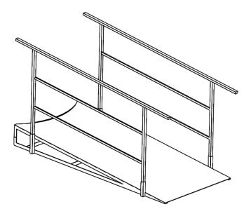
Figure 10.- Platform access ramp with safety rails.
