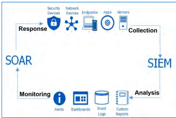
Fig. 7. SOC Functional Components
