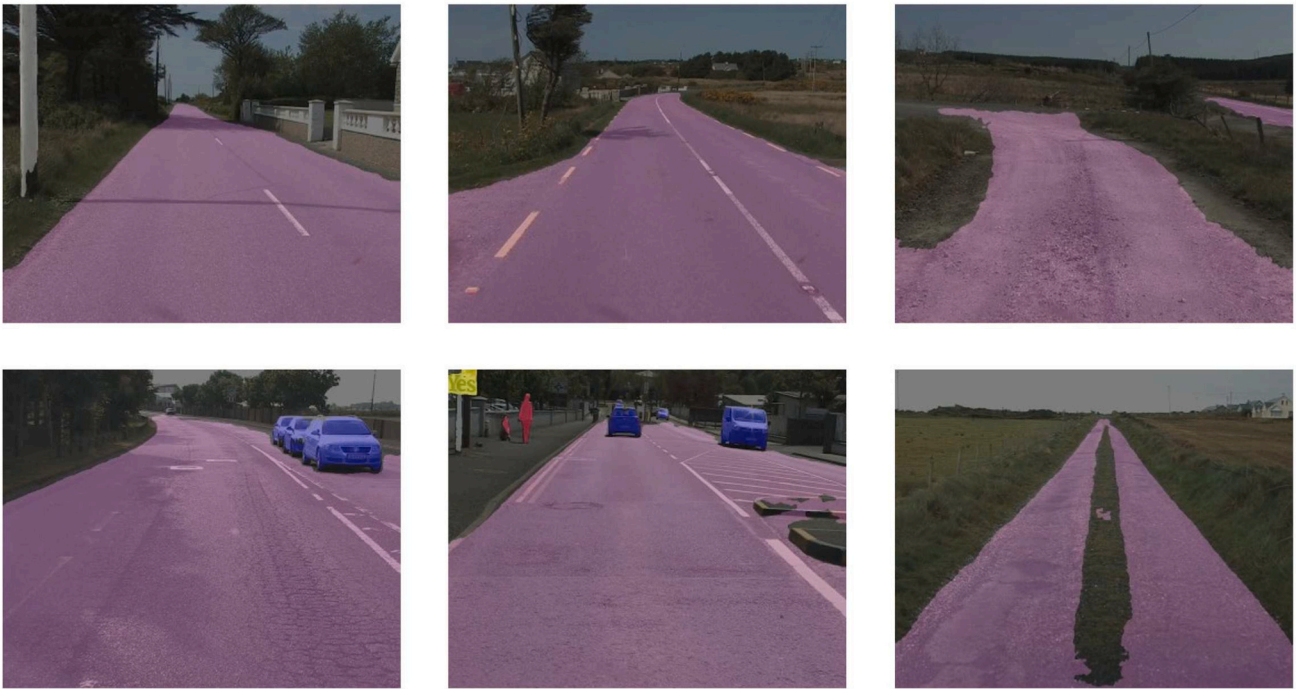
Fig. 10. Sample segmentation mask overlaid on original images from test dataset using the Model DeepLabV3 b trained on IrishRoadSurvey-1 and Cityscape dataset with 7 classes.
