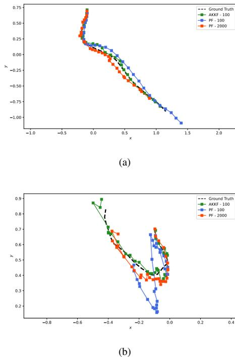
Fig. 2: BOT tracking of a moving target in two dimensions of Trajectory-1 (a) and Trajectory-2 (b) using the quartic kernel-based AKKF with 100 particles; the PF with 100 particles; and the benchmark performance of the PF with 2000 particles. The physical unit on the X-axis and Y-axis is the ‘metre’.
