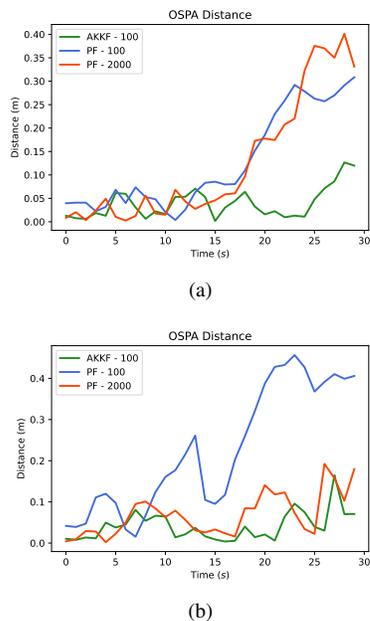
Fig. 3: Performance of BOT tracking of a moving target in two dimensions of Trajectory-1 (a) and Trajectory-2 (b) using the OSPA [13] distance.
