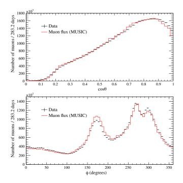
FIG. 2. Zenith  $(\theta)$  and azimuthal  $(\phi)$  dependence of the muon rate at the SK site. Reconstructed directions of the muons from the data (black points) are overlaid with the muon flux at the SK site calculated by the MUSIC code (red lines). Muon flux distributions are normalized to the data.  $\phi=0$  corresponds to the direction from east to west.
