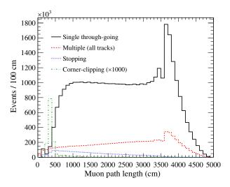
FIG. 1. Distributions of path length  $L_{\mu}$  for single through-going (solid), multiple (dashed), stopping (dotted), and corner-clipping (dot-dashed) muons. The distribution of corner-clipping muons is scaled by a factor of 1000.
