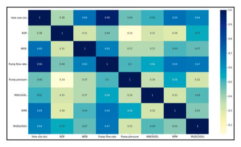
Fig. 12. Correlation matrix for the selected parameters for modeling.
