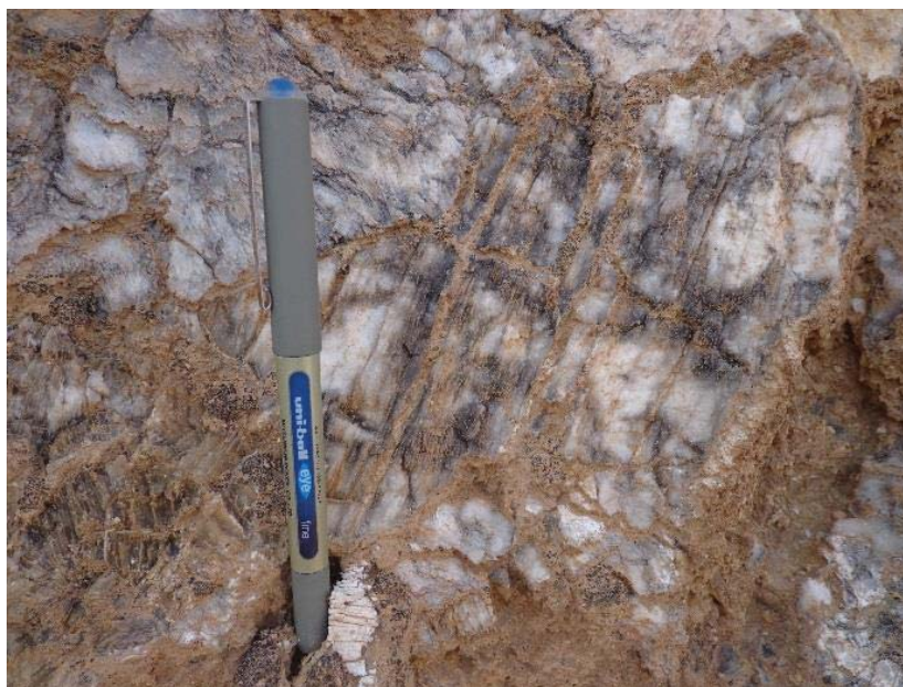
Fig. 2: Field photo shows bituminous gypsum in the Fatha Formation near Hit area
