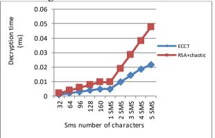
Figure 3. Comparing decoding time in ECCT + RSA based on the number of SMS characters.
