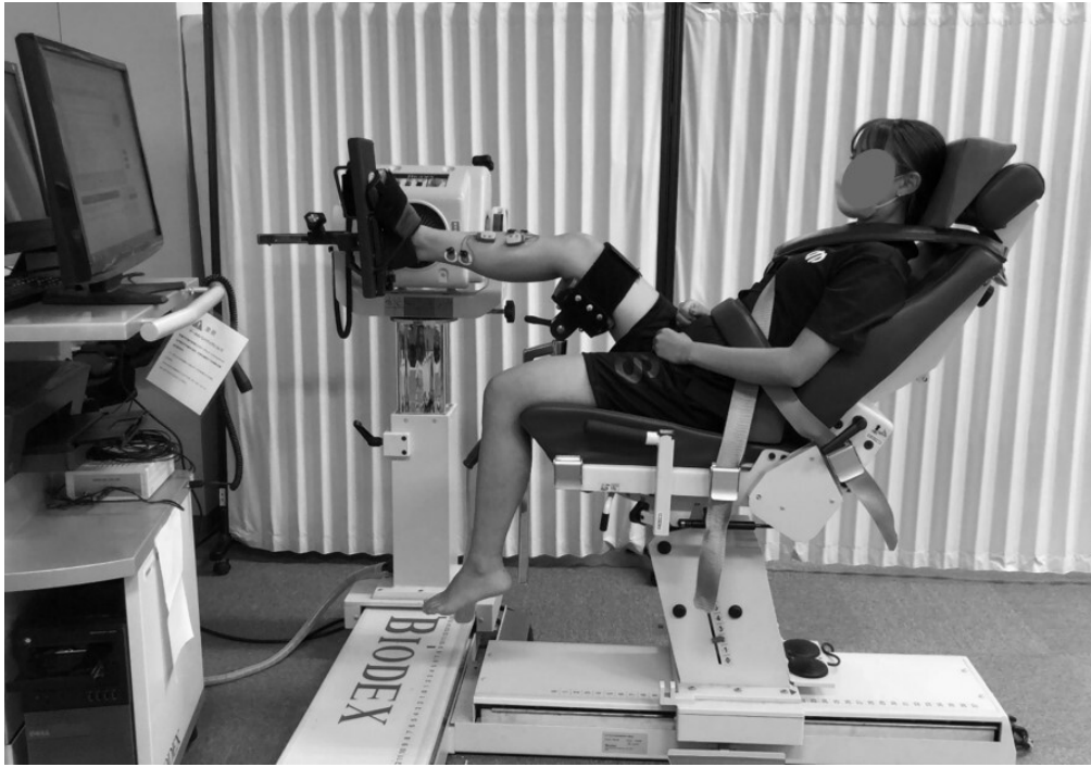
Figure 2. Testing position for the maximum voluntary isometric contraction testing and torque control testing
