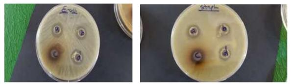
Figure 4. Antibacterial test against *Esherichia coli* and *Staphylococcus aureus*, for nanocomposite P<sub>2</sub> with different weight of Ag, a= P<sub>2</sub>/Ag 1%, b= P<sub>2</sub>/Ag 3%, c= P<sub>2</sub>/Ag 5%, d= P<sub>2</sub>/Ag 7%.
