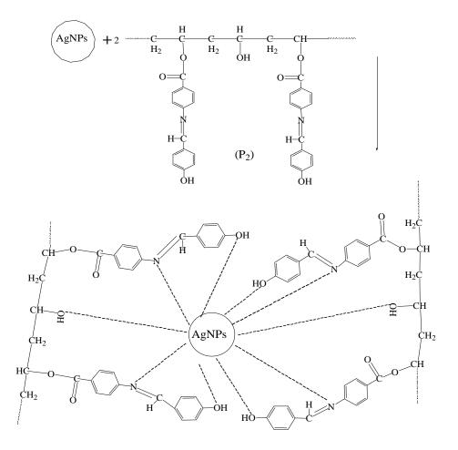
(Nanocomposite (NCs) from Ag nanoparticles and P<sub>2</sub>) Figure 2. Process of synthesizing nanocomposite (NCs) from Ag nanoparticles and P<sub>2</sub>
