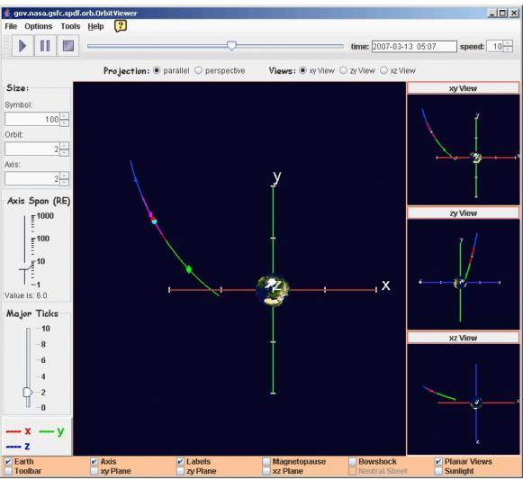
Positions of spacecraft on Mar 13 2007 near 5:08 UT onset time. Scale is marked at 4 R<sub>e</sub> intervals and dots are THEMIS C, D, B, A, and E, from lower right in main plot.
