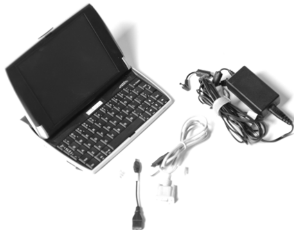
Figure E2. The Netbook Pro with AC adapter, USB cable, and RS 232 cable.
