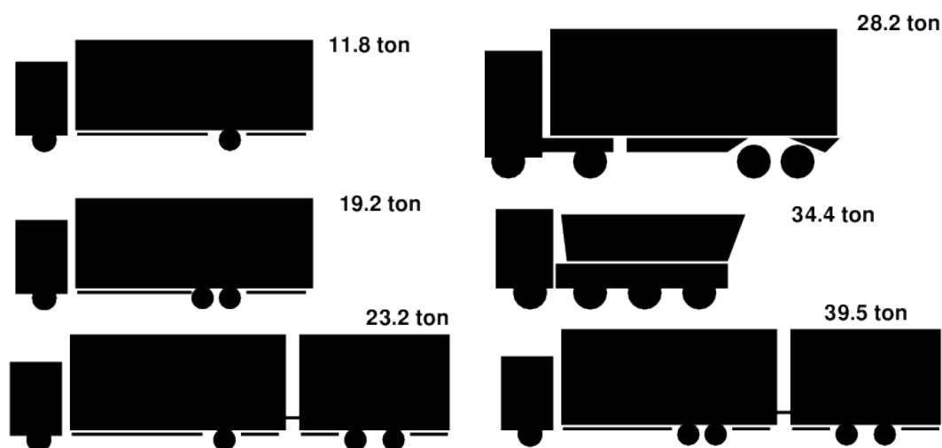
Figure 4.6 Average (on-road) vehicle weight of different heavy-duty truck configurations in the Netherlands, derived from the WiM system (source: TNO).
