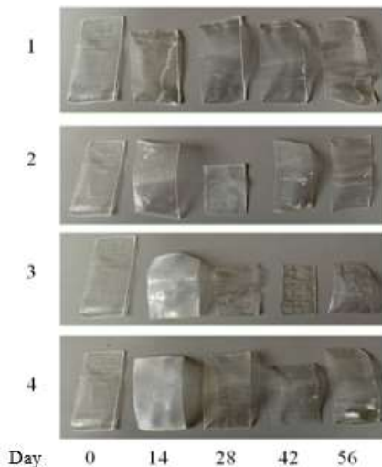
Fig. 6. Appearance of PLA tapes before and after exposure in different types of soil at different temperatures: 1 – humus, 23 °C; 2 – humus, 8 °C; 3 – chernozem, 23 °C; 4 – chernozem, 8 °C
