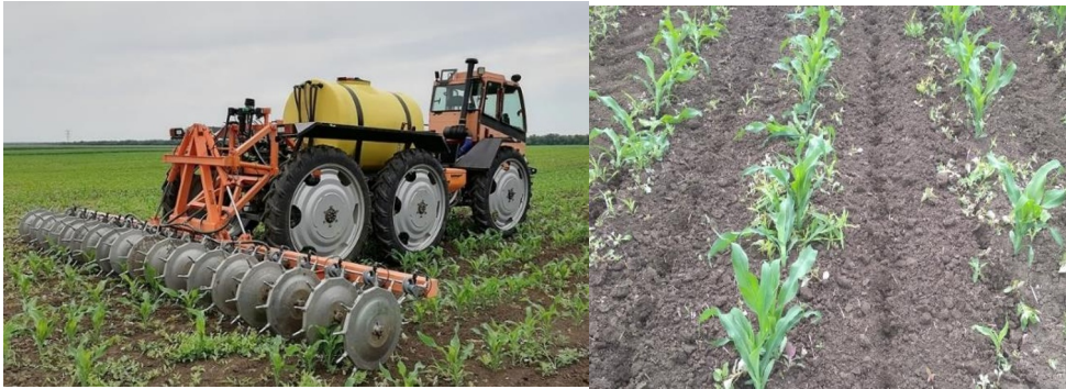
Fig. 6. Operation of the “Tuman-2M” multi-injector from LLC “Pegas-Agro” when applying CAM: work with corn on narrow support wheels, traces of injection needles
