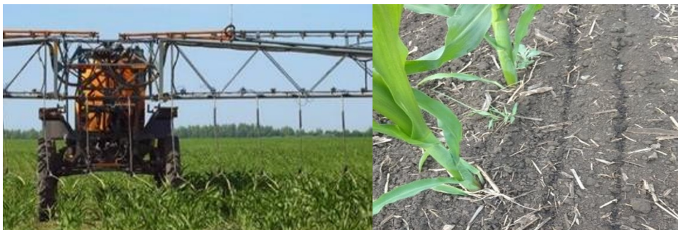
Fig. 5. Processing of corn with liquid fertilisers CAM-32, CAM+S with extension hoses on the “Tuman-2” sprayer, traces of CAM on the soil after passage
