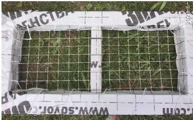
Fig. 3. Bioplate construction: 1 - frame, 2 - mesh
