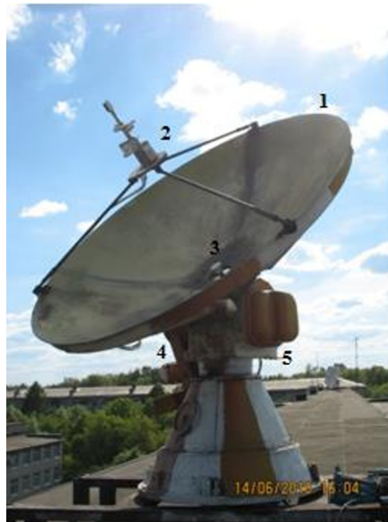
Fig. 4. Antenna system of modern complex: 1 - Straight-focus mirror with a diameter of 2400 mm; 2 - Multichannel two-mode irradiator with removed weather protection; 3 - Multifrequency waveguide microwave calibrator; 4 - Angular actuator; 5 - Azimuthal actuator.
