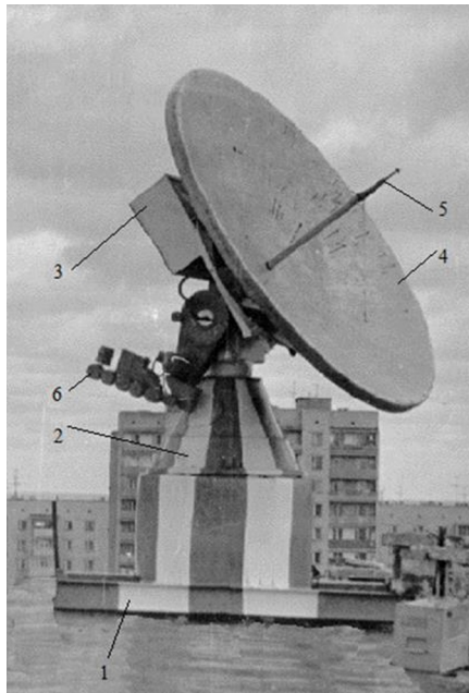
Fig. 2. PARLS antenna system: 1 - supporting frame; 2 - antenna column; 3 - location of AC and PC; 4 - parabolic reflector; 5 - an irradiator; 6 - counterweight.
