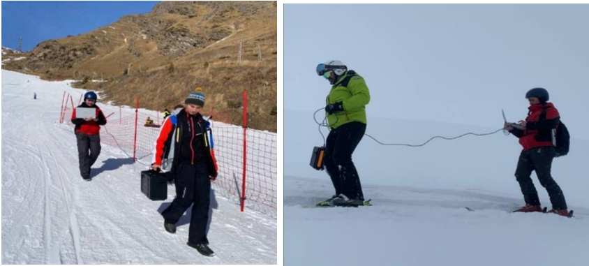
Fig. 2. Left - georadar profiling of the left part of the rollout in the area of Azau station (2350 m). Top-down movement. Photo by Zhukova E.D. On the right - georadar profiling in the area of pit No. 2 (Small Azau ) using ski equipment to move along the snow cover. Photo Lisachenko E.S.
