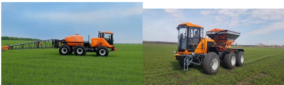
Fig. 6. Technological self-propelled complexes “Tuman” from “Pegas-Agro” LLC (Samara, Russia): a) - rod sprayer, b) - spreader-distributor of solid mineral fertilisers
