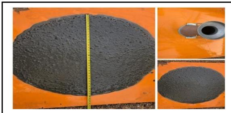
Figure 6: The slump flow test.
