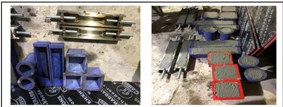
Figure 4: Sample molding for each examination model.
