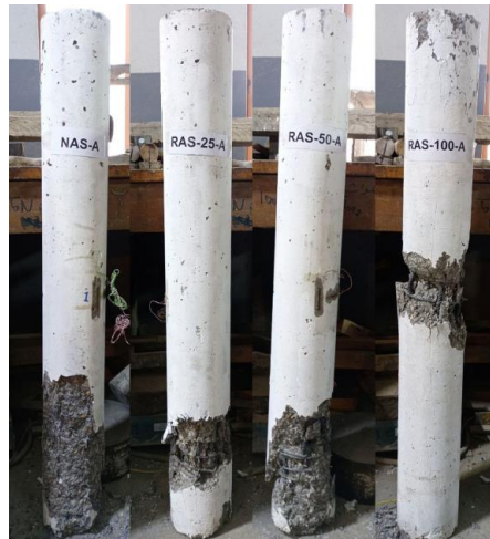
Figure 4: Failure patterns of columns with a spiral reinforcement.
