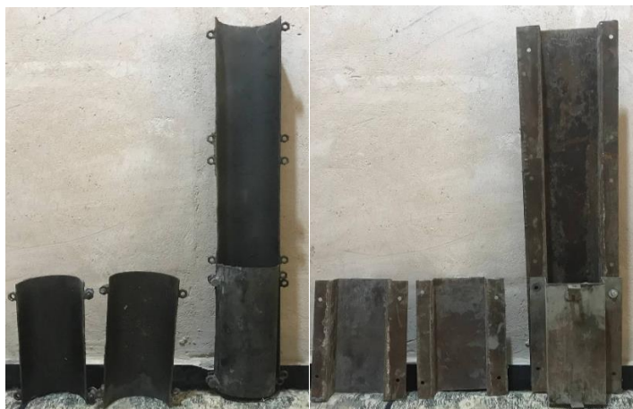
Figure 4: Square and circular iron molds.
