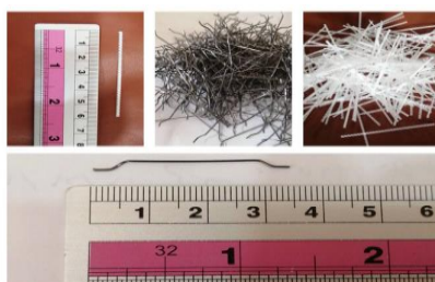
Figure 1: Hooked end steel fiber and polypropylene.
