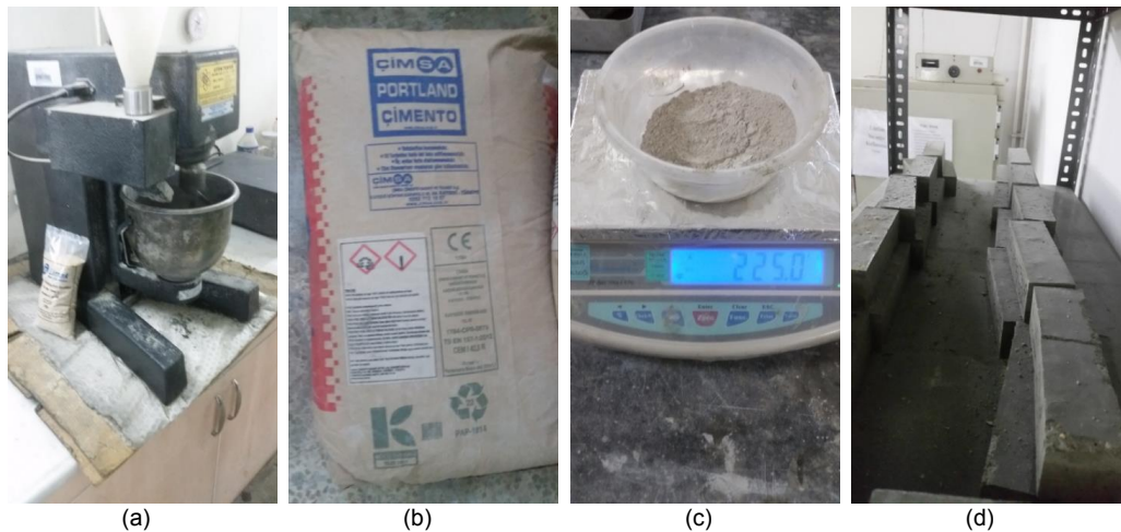
Figure 1: a) Hobart mixer, (b) Ordinary Portland cement Type I, (c) Electronic scales used to measure material weights, (d) Mortar specimens.
