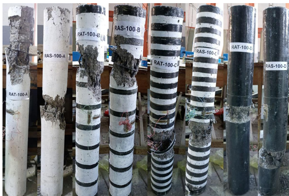
Figure 5: Failure patterns of columns with tied reinforcement.
