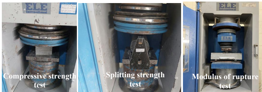
Figure 3: Mechanical properties tests.
