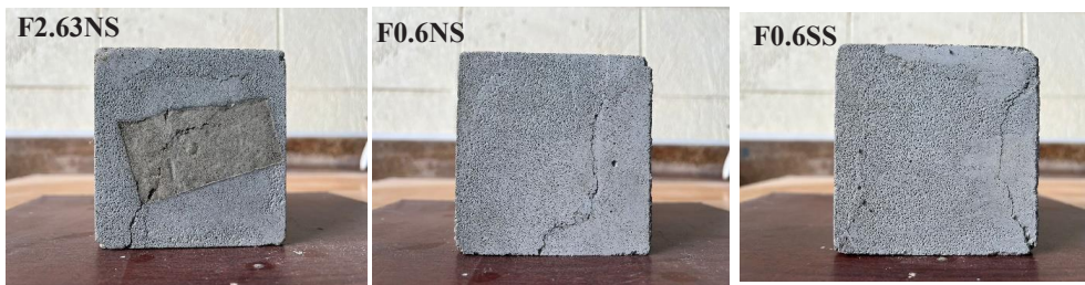
Figure 7: Shape of failure under compression load.
