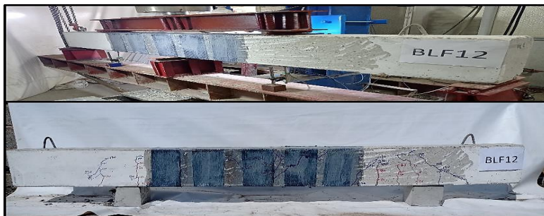
(b) Crack patterns in the tested extended continuous beams at the failure stage (BLF12).
