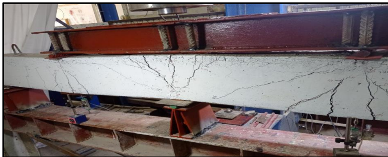
(a) Cracks pattern of CB.
