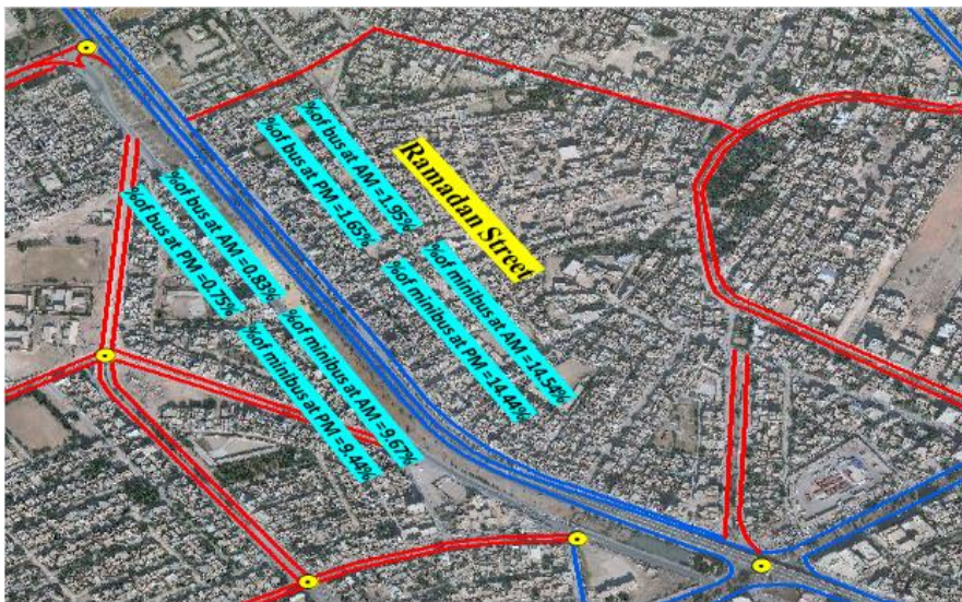
Figure 9: The average ratio values of bus and Minibus in GIS for Ramadan Street at AM and PM.
