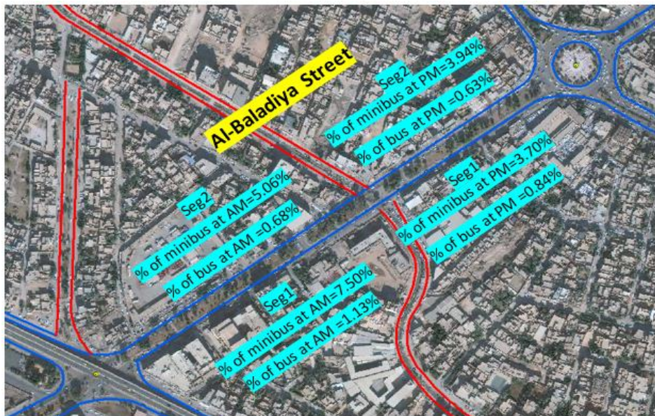
Figure 13: The average ratio values of bus and Minibus in GIS for Al-Baladiya Street at AM and PM.
