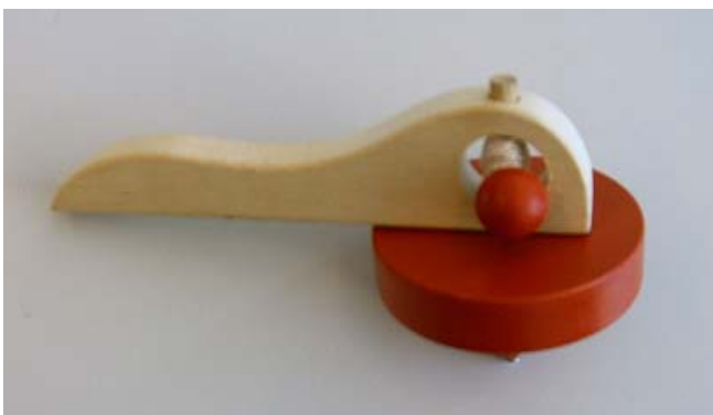
Figure 12. The kind of top tested from which the paint contained lead levels above the allowed level.
