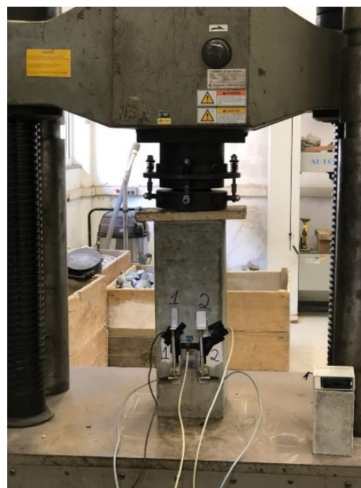
Figure 14. RC Column with sensors connected to the QuantumX MX840B data system.
