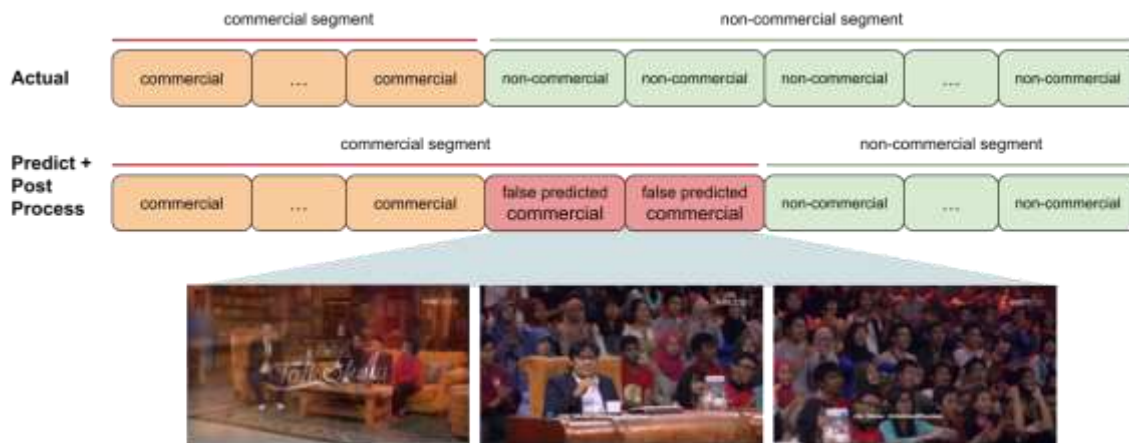
Figure 7 Inaccurate shot level detection at the edge of a segment
