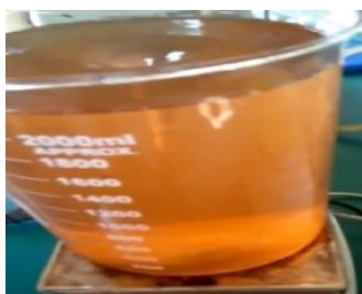
Fig. 5. Solution of cobalt acetate with the plant extract during cobalt nanoparticles synthesis.
