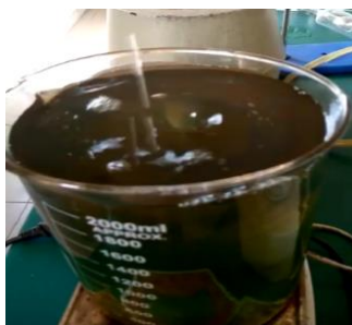
Fig. 6. Addition of Sodium hydroxide on the cobalt acetate and plant extract during synthesis of cobalt nanoparticles.
